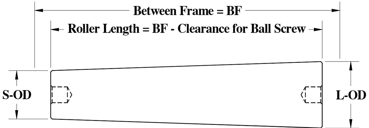
Blind bore tapered rollers are ideal for light to medium duty gravity roller curves used in corrosive, wash down or food handling environments. To order these rollers specify the material the roller is to be manufactured from, the outside diameter of the large and small end of the roller, the between frame dimension and the ball screw size.
