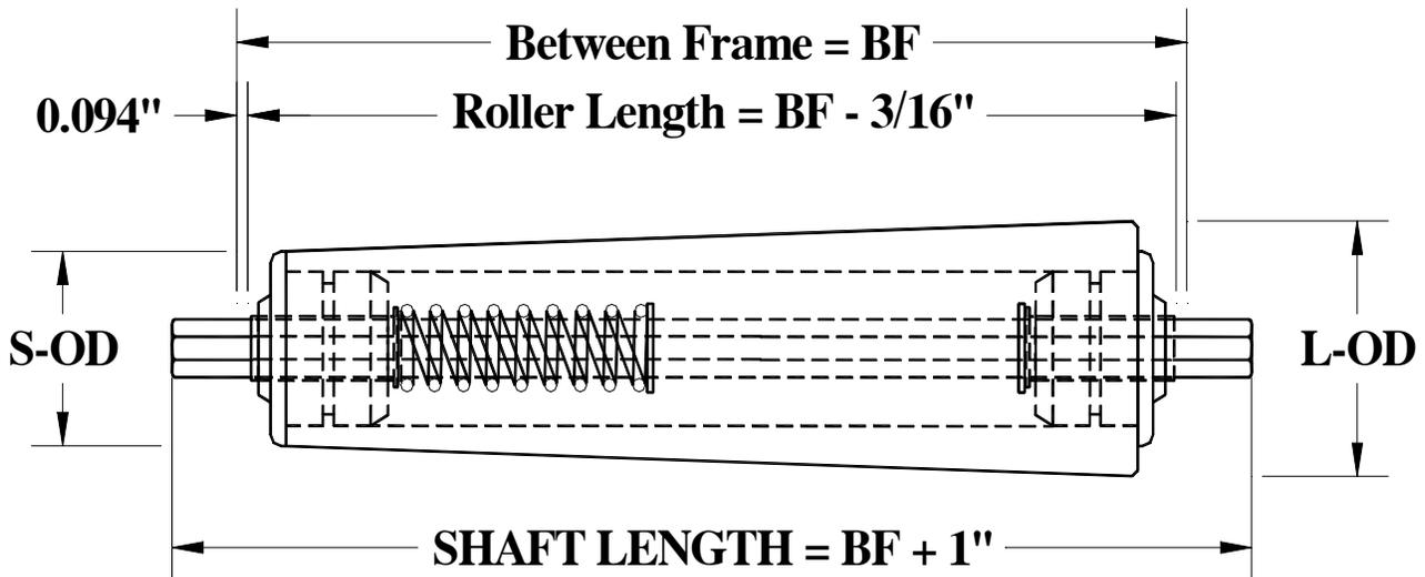
Spring loaded or pin retained tapered rollers are ideal for medium to heavy duty gravity roller curves used in corrosive, wash down or food handling environments. To order these rollers specify the material the roller is to be manufactured from, the outside diameter of the large and small end of the roller, the between frame dimension and the shaft size and material type.
